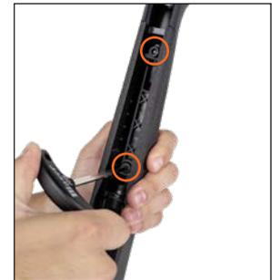
Loosen the two forearm tip mounting screws using an Allen key (size 5) and remove them with the lock washers.
